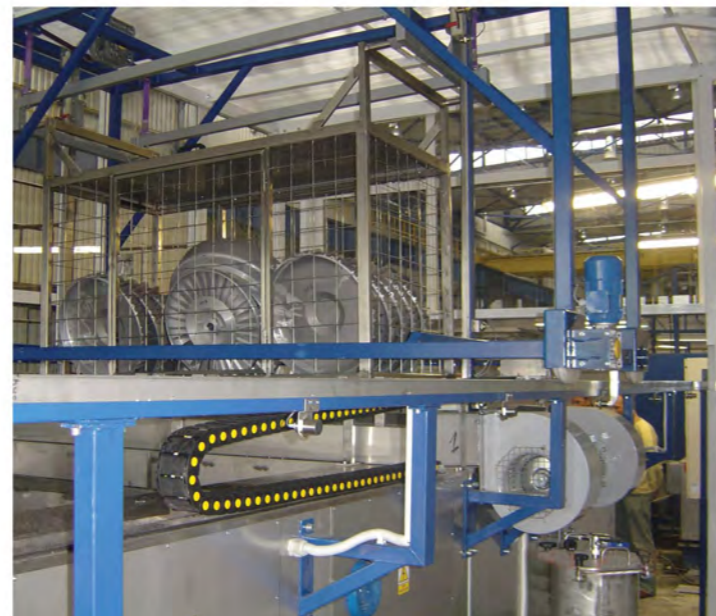
Line for surface preparation of aluminium and steel workpieces before painting.
