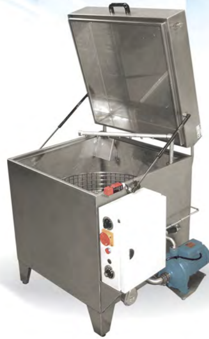
Spray cleaning station w/ a rotary basket.
