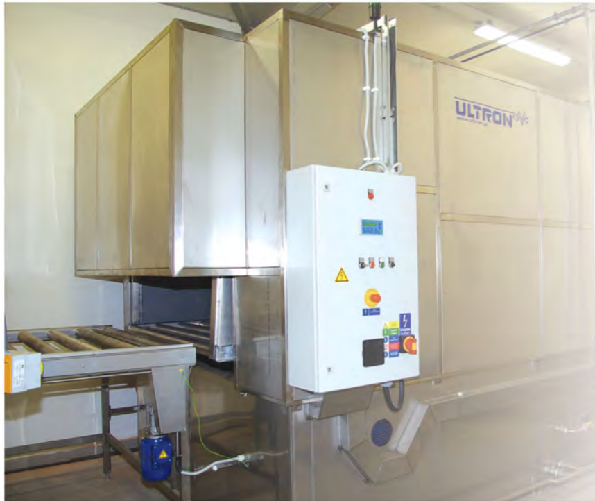
Line for surface preparation before powder coating.
